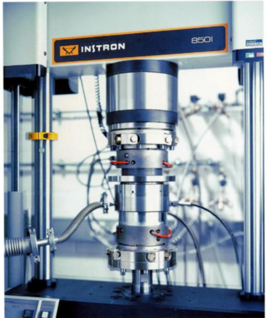
Test set-up to determine helium tightness.
